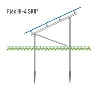
Crystalline modules: two rows, vertical three rows, horizontal
